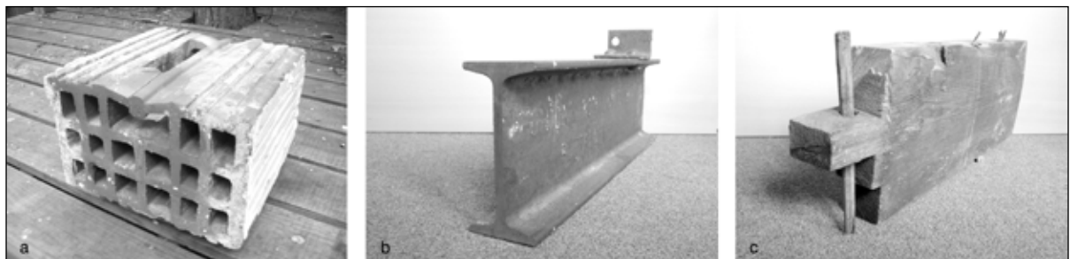
Fig. 4. Structural remnants for in-class assessment: (a) terra cotta foundation block (1938); (b) steel I-beam (1913); (c) wood joist and connection (1810).
