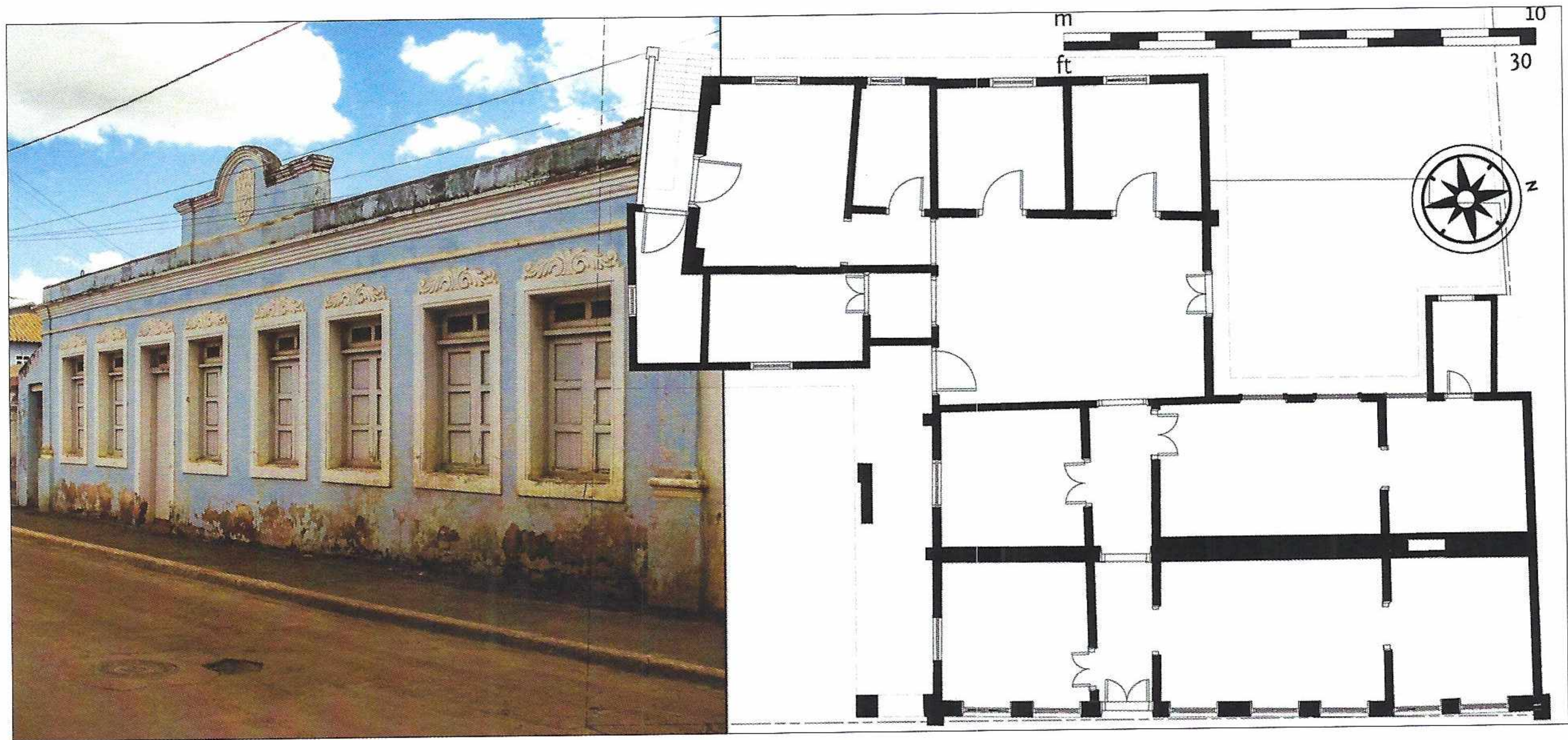
Fig. 6. Blue house, built 1926. (Photograph and plan by the author, as surveyed in 2009.)
