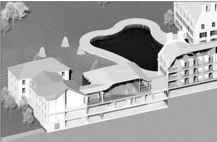
Fig. 10. Partial axonometric section of the proposed addition to the Carolina Inn, December 5, 2008 (Meghan Roller, University of Illinois School of Architecture).
